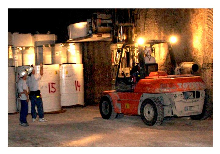
WIPP personnel place "super sacks" of magnesium oxide on the top of waste columns during underground waste disposal operations.
